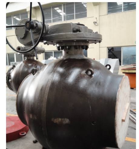
WB(焊接连接) WB(Welding connection)
